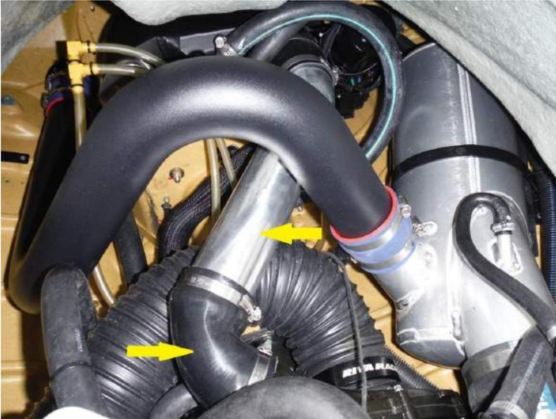
20. Install supplied straight reducer silicone coupler onto the throttle body. Loosely place two supplied hose clamps over coupler on throttle body (smaller one goes on the throttle body) and one over the coupler at the intercooler. Install the hard pipe that runs from the throttle body to intercooler. Work the angle of the pipe until it lines up properly. Tighten all hose clamps on intercooler piping and then the clamps at the waterbox.
