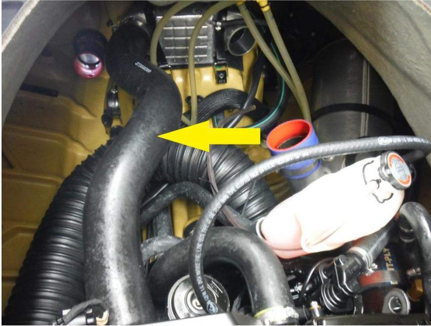
10. If applicable (2013+ models) remove the intercooler bleeder line.
