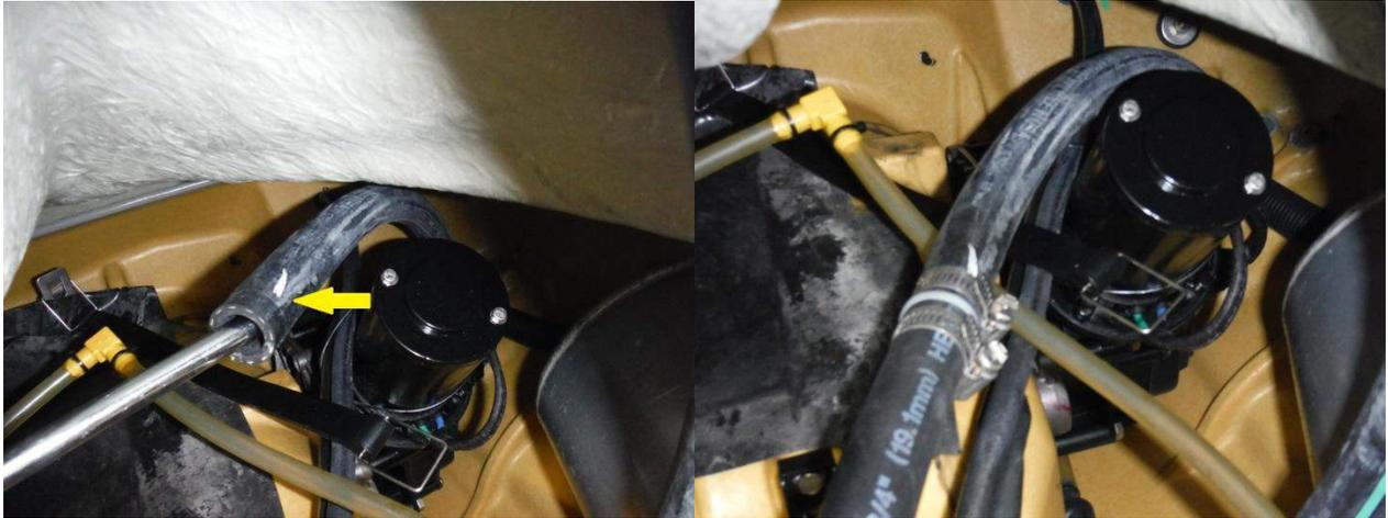
18. Install exhaust tube, OEM exhaust hose or aftermarket pipe from the waterbox to your exit outlet. You can leave the clamp on the waterbox loose for now to allow for intercooler pipe fitment.
