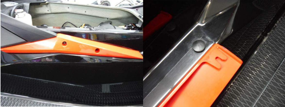
2. Remove top grab handle cover by removing the two Torx T-30 screws and two plastic push pins.
