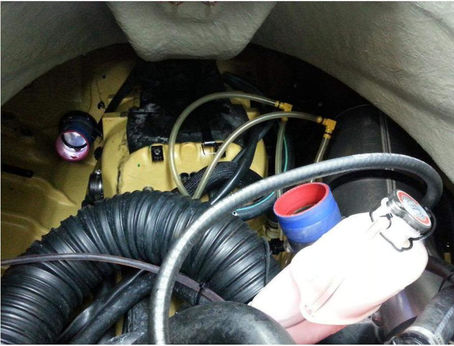
14. Find the 1/4" bleed hose that was originally attached to the top right of the OEM intercooler and install the supplied plug. Place the OEM hose clamp on line and secure it with a zip tie.
