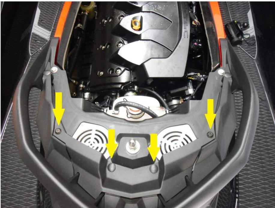
3. Remove second rear grab handle cover by removing the Torx T-30 screw by two hook, two plastic push pins on top, and one plastic push pin on each side.
