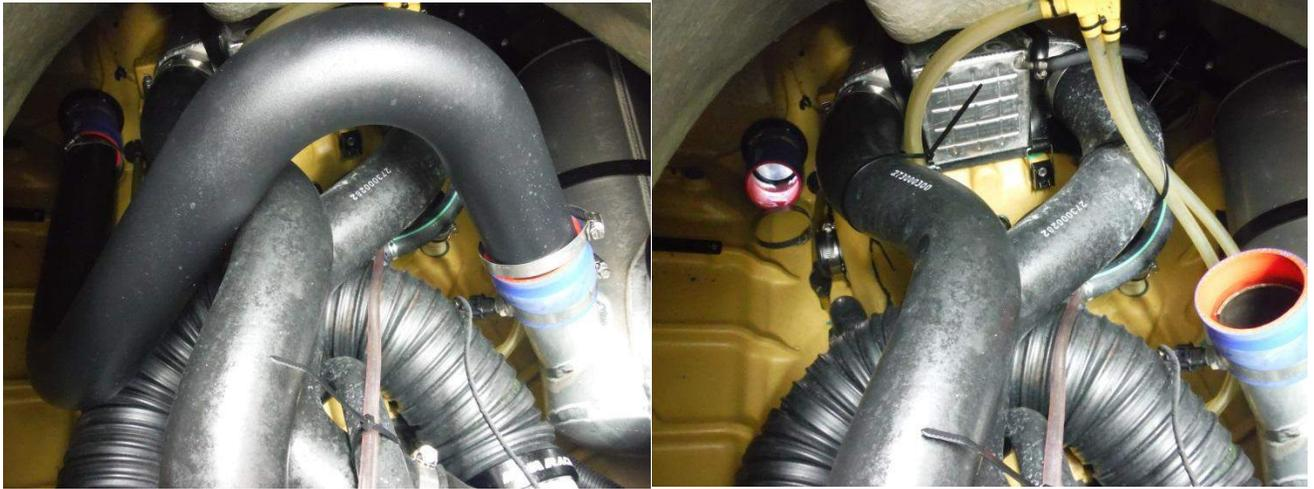
8. Remove supercharger-to-intercooler hose.
