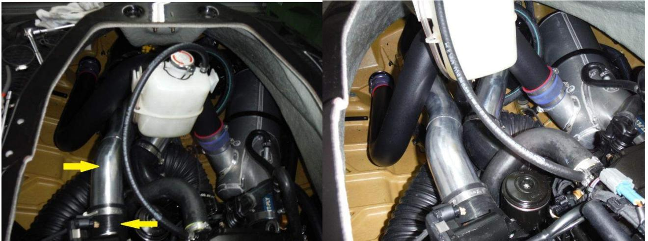
21. Install rear grab handle, coolant overflow tank, grab handle covers, and side engine bay plastic covers by following steps 1 through 6 in reverse order.
