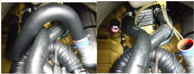
8. Remove supercharger-to-intercooler hose.
