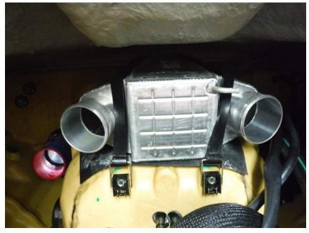
12. Identify and take note of the in and out water lines going to the intercooler. Water in line comes from the T located closest to the transom and goes to the bottom of the intercooler. Water out line comes from the intercooler and goes to the back of the hull to a T close to the OEM flush port.
