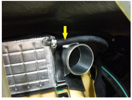
11. Remove the two intercooler straps.
