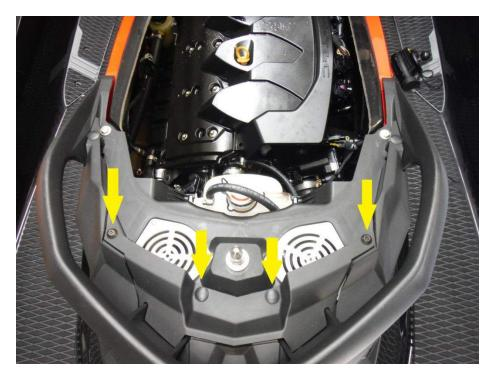
3. Remove second rear grab handle cover by removing the Torx T-30 screw by two hook, two plastic push pins on top, and one plastic push pin on each side.
