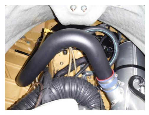
19. Install supplied 90 degree reducer silicone coupler onto the supercharger. Loosely place two supplied hose clamps over coupler on supercharger (smaller one goes on the supercharger) and one over the coupler at the intercooler. Install the hard pipe that runs from the supercharger to intercooler. Work the angle of the supercharger coupler and pipe until it lines up properly. Tighten all hose clamps.
