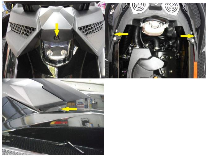
4. Remove coolant bottle overflow tank from grab handle by pushing in on both side clips of the bottle and pull up
