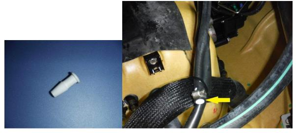
15. Install supplied brass barb fittings into the intercooler. The top should have the 90 degree and the bottom should have the straight fitting. Install the 90 degree fitting first.
