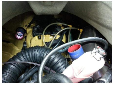
14. Find the ¼" bleed hose that was originally attached to the top right of the OEM intercooler and install the supplied plug. Place the OEM hose clamp on line and secure it with a zip tie.
