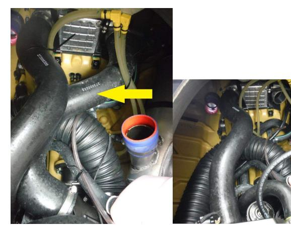
9. Remove intercooler-to-throttle body hose.
