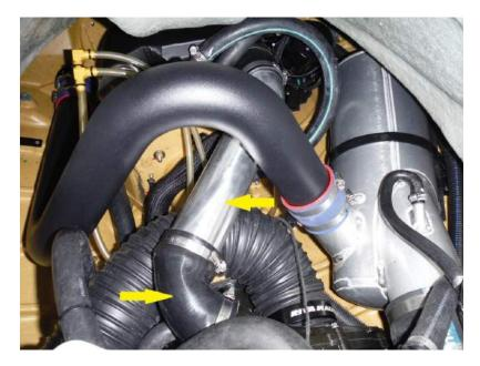
20. Install supplied straight reducer silicone coupler onto the throttle body. Loosely place two supplied hose clamps over coupler on throttle body (smaller one goes on the throttle body) and one over the coupler at the intercooler. Install the hard pipe that runs from the throttle body to intercooler. Work the angle of the pipe until it lines up properly. Tighten all hose clamps on intercooler piping and then the clamps at the waterbox.
