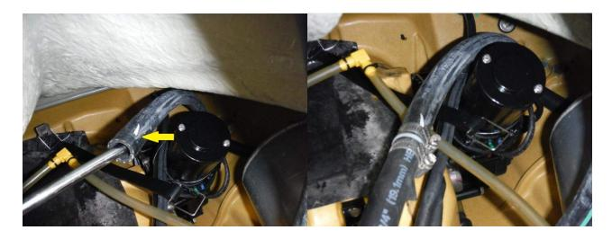
18. Install exhaust tube, OEM exhaust hose or aftermarket pipe from the waterbox to your exit outlet. You can leave the clamp on the waterbox loose for now to allow for intercooler pipe fitment.
