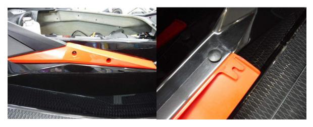
2. Remove top grab handle cover by removing the two Torx T-30 screws and two plastic push pins.
